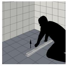
2. Remove the grating plastic locks from the sides of the grating and insert the LED unit making sure that the LEDs are facing toward the center of the grating while the angled top faces upward allowing water to drain freely.
